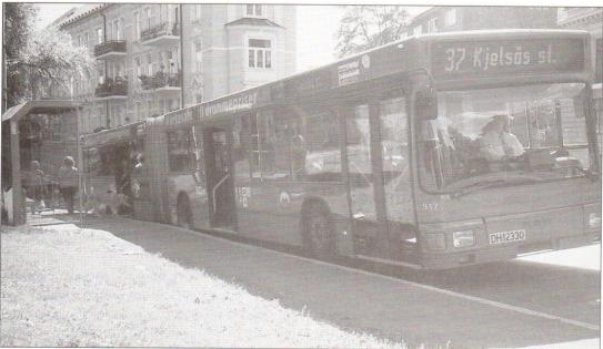
**Low floor buses** with entrance from bus stops with highlevel platforms ( at the bottom) are more in line with universal design because:
